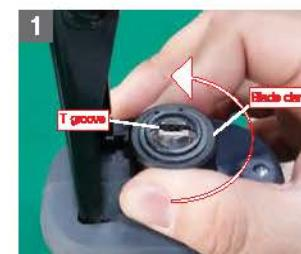
▶ Rotate the blade clamp sleeve in the direction of the arrow fully (90°)
