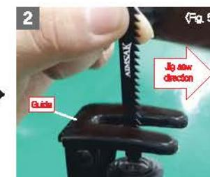
▶ While holding the blade clamp in the rotated position, insert the Jig saw blade into the blade clamp as far as it will go. (Refer to Fig. 5)
